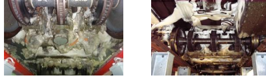
Figure 1. Snow and ice accumulation on the bogies of high-speed trains.
